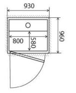
Hole through floor: 930x960 mm Platform: 800x580 mm Doors: 800 mm Load: 250 kg
